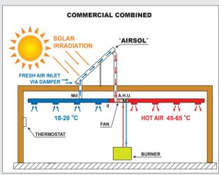
It can be used either as the only source of heating or as a back-up one. It can be combined with any oil or natural gas boiler (burner).
