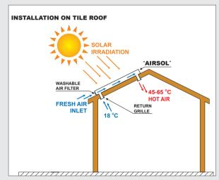
Installation on **inclined roof** facing south, south east and south west
